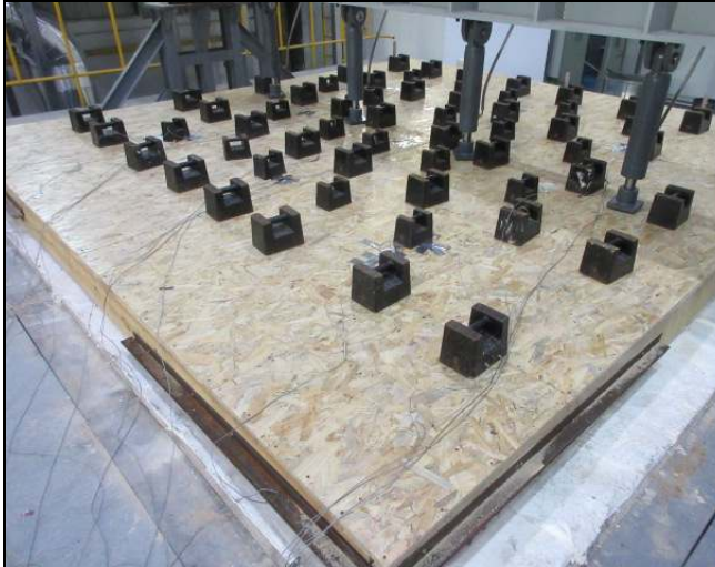
Photo 13: The unexposed face before the test (Distribution of the weights)
