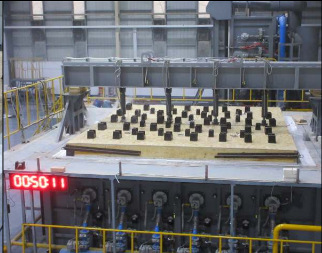
Photo 14: The unexposed face of sample (After test duration of 50 minutes)
