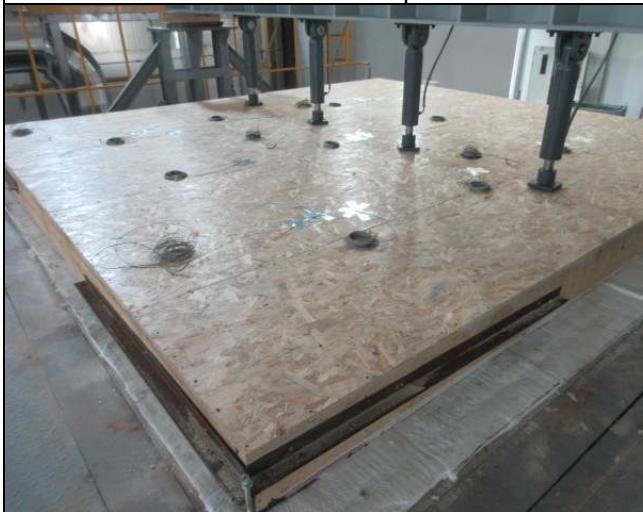
Photo 11: The unexposed face before the test
