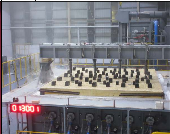
Photo 16: The unexposed face of sample (After test duration of 90 minutes)
